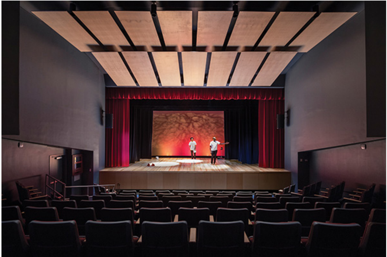
Billie Holiday Theater upgrades included new seating, enhanced lighting, symmetrically reshaping interior walls, expanding the stage with sprung-maple flooring, and adding acoustical panels to the ceiling.
